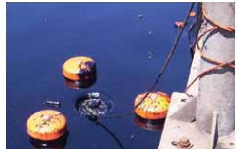
HIGH VOLUME FUEL OIL SKIMMER SPILLAGE.
