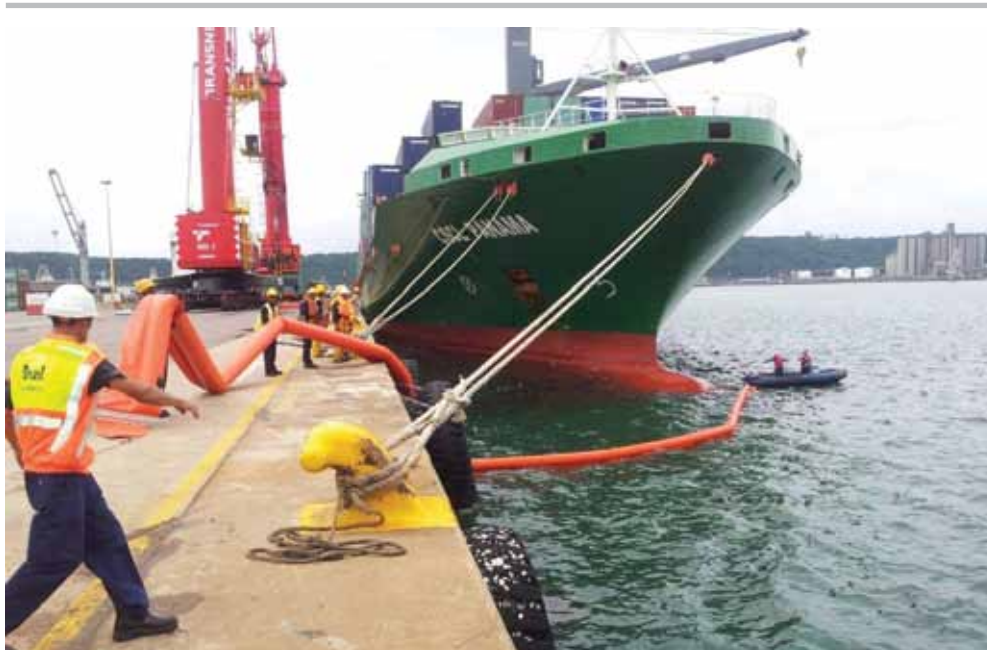
POLLUTION PREVENTION BOOMING OF VESSEL IN PORT
